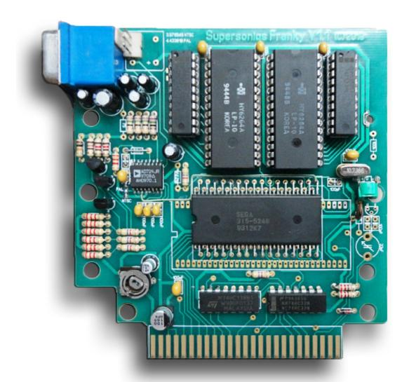
The photo above can be used as a reference for mounting. The value of all components are on the pcb itself, just follow what's printed. Some pcb's have blurred values on the text of the electrolytic capacitors. Please look below for the correct values of these capacitors:
