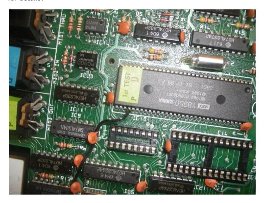
The other end of the wire needs to be connected to PIN 9 of IC2 (the IC will read something like 74LS04). See picture below.
